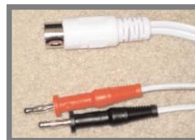
Red/black leads for the body pads, white cord: body
